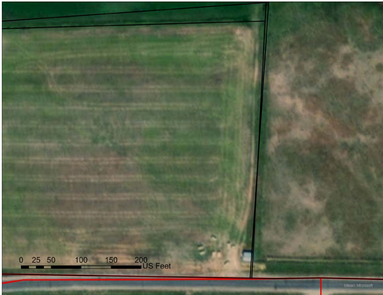
Figure 1. Small slivers created from the union between the 2019 and 2009 data. The small red sliver on the bottom left corner shows land previously labeled as irrigated land in 1976 and a road in 2019. The sliver running north and other black slivers represent no change, but the polygons to represent these agricultural fields shifted slightly over time.
